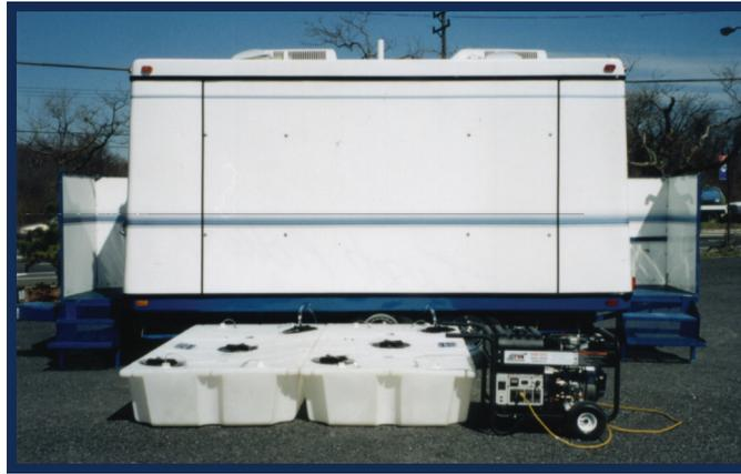
Water and electric can be supplied by CALLAHEAD with 2-300 gallon fresh water tanks and a 100 AMP generator.
