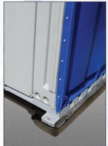
**DESIGN FEATURES:** Thermoformed from tough, impact resistant high molecular weight, high density polyethylene. • Serves as a drip tray to contain water and cleaning solutions during servicing. • Fluids drain towards the rear of the tray to a convenient pump out location. • The trays have a peripheral lip that guides fluids into the pan. • Will fit beneath most portable restrooms. • Support ribs for extra strength beneath the "runners" to raise them out of fluids between servicing.
